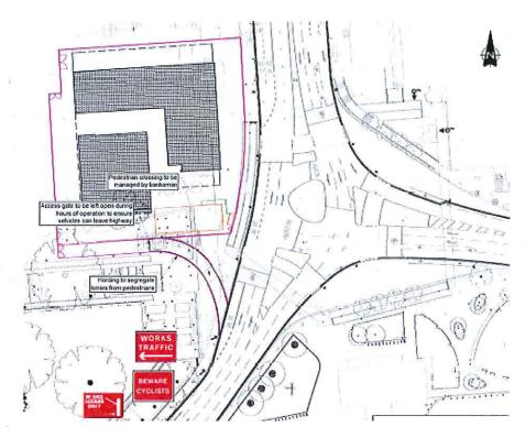
All vehicles will turn within the Site in order to minimise disruption to other road users. A plan showing the designated construction route is illustrated in the Travel Plan
